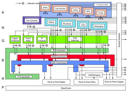
Figure 2: Telecommunications service elements
